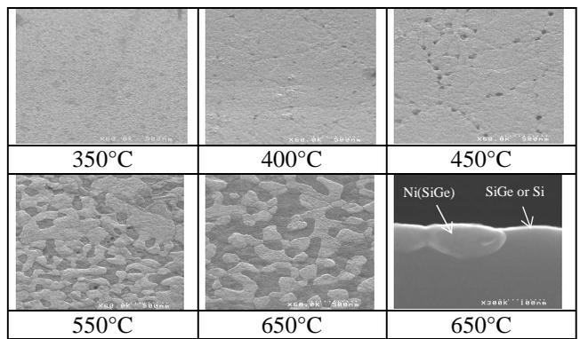
Figure 2 : top-view and cross sectional SEM micrographs of Ni9nm/Si<sub>0.75</sub>Ge<sub>0.25</sub> 25nm samples annealed at different temperatures. Top-view pictures are tilted at 60°
