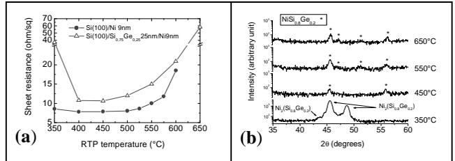
Figure 1 : sheet resistance (a) and XRD  $\theta/2\theta$  patterns (b) as a function of Rapid Thermal Annealing temperature of Ni 9nm/Si<sub>1-x</sub>Ge<sub>x</sub> (x=0 and 0.25) 25nm films. RTA is performed for 60s in an Ar ambient.
