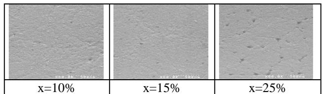
Figure 3 : top-view SEM micrographs (tilted at 60°) of Ni9nm/Si<sub>1-x</sub>Ge<sub>x</sub> 25nm samples annealed at 450°C for 60s in Ar ambient for different x values
