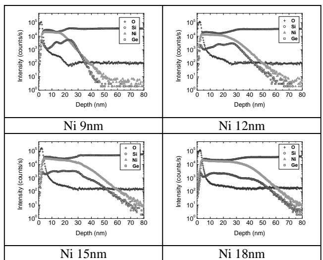
Figure 4 : SIMS profiles for Ni/Si<sub>0.8</sub>Ge<sub>0.2</sub> 25nm samples annealed at 450°C for different Ni thickness
