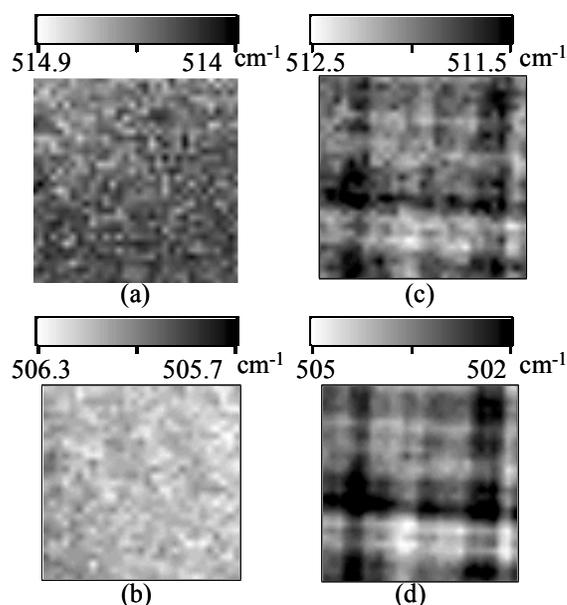
Fig.2 Raman mapping images of Si-Si mode of (a) strained-Si on SGOI (b) SiGe in SGOI (c)strained-Si on virtual substrate and (d) SiGe in the virtual substrate.
