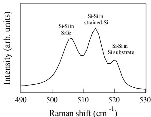
Fig.1 The typical Raman spectrum obtained from the strained-Si on SGOI.
