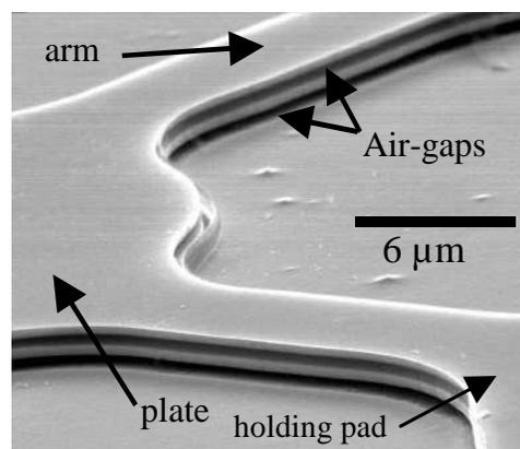
Figure 2 SEM of the circular plate and two supporting arms
