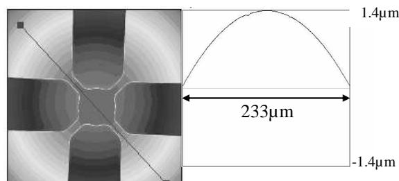
Fig. 3 WLI measurement on a InP membranes symmetrically supported by four arms
