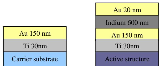
Fig. 2 Metalisations evaporated on the carrier substrate and the active structure.
