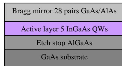
Fig. 1 GaAs-based VECSEL structure for bonding
