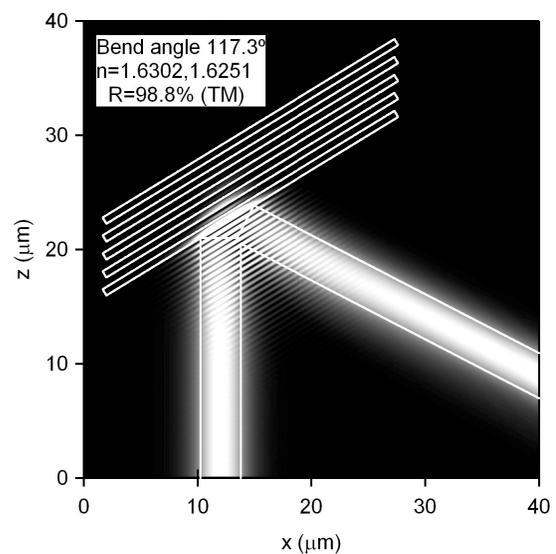
Fig. 1. Multi-air trench bend in LIC waveguide material system for  $\lambda=1.33\mu\text{m}$ .
