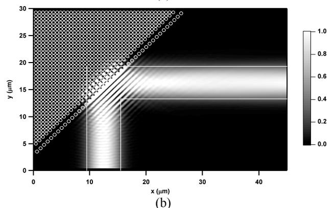
Fig. 2. Air hole photonic crystal bend in silica waveguide material system. (a) Power ratio of reflected light to incident light as a function of wavelength for the initial structure (dashed line) and the structure after optimization process (solid line). (b) Magnitude squared time averaged electric field for  $\lambda=1.55\mu\text{m}$  for the final optimized geometry.
