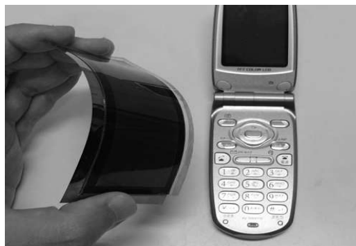
Figure 3 A name-card size full-plastic DSSC.
