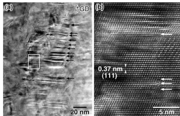
**Figure 3.** High resolution TEM image of as-prepared CdTe layer electrodeposited from acidic bath at  $-0.37$  V.
