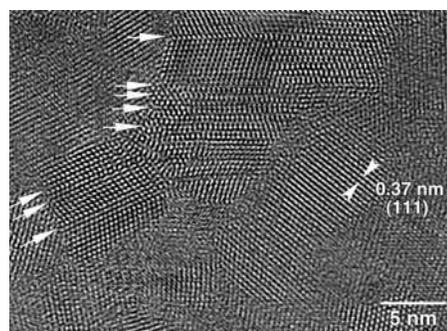
**Figure 2.** High resolution TEM image of the same layer shown in Fig. 1. White arrows indicate planar defects on {111} plane.
