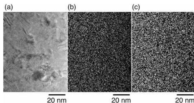
**Figure 4.** (a) High resolution scanning TEM image and (b, c) elemental distribution map of the same layer shown in Fig. 1; (b) Cd and (c) Te.
