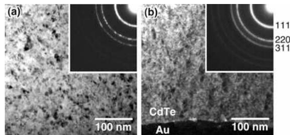
**Figure 1.** TEM images and corresponding SAED patterns of as-prepared CdTe layer electrodeposited from basic bath at  $-0.70$  V; (a) plan-view, (b) cross-sectional view.
