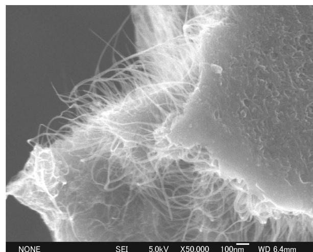
Figure 2. SEM image of the functionalized SWNTs.
