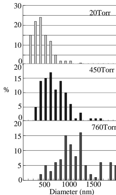
Fig.2 Size distribution of Cu particles produced in He gas on d-CNTs.
