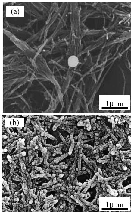
Fig.1 SEM images of copper particles on (a) as-grown (d-CNTs) and (b) ultra-sonicated carbon nanotubes (r-CNTs).
