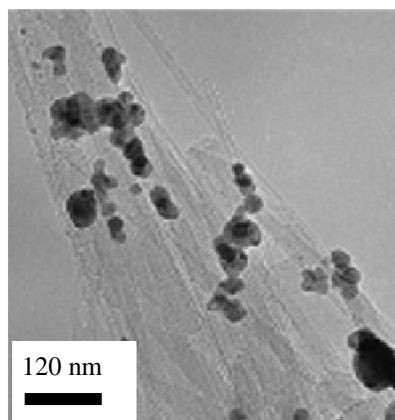
Fig.3 A TEM image of copper nano particles deposited on r-CNTs.
