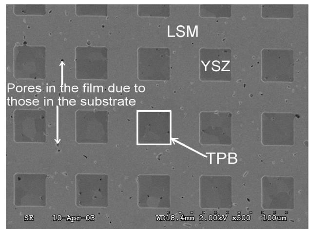
Figure 1. SEM of an LSM electrode on YSZ
