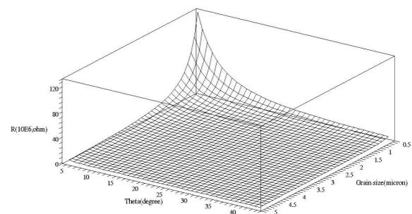
Figure 2. Total resistance as a function of grain size and the angle (which determines the neck radius) for the case with  $\rho_s = 14520$  ohm.cm,  $\rho_g = 76$  ohm.cm.
