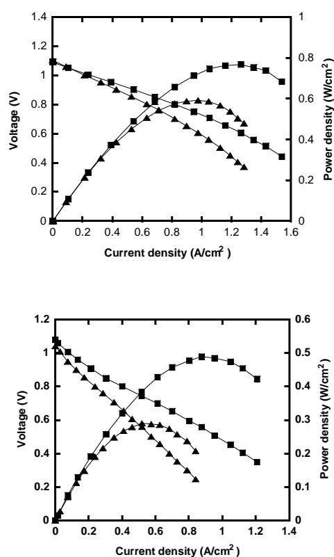
Fig. 1 Cell performance curves at 973 K (▲) and 1023 K (■) in  $\text{H}_2$  (top curves) and n-butane (bottom curves).
