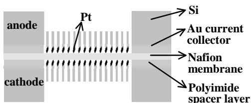
**Figure 1.** Schematic diagram of silicon-based MEA.
