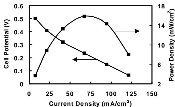
**Figure 2.** IV and power density data curves for silicon-based microfuel cell with formic acid as a fuel under forced feed conditions. Anode side: 10 M formic acid at a flow rate of 0.5 ml/min, Cathode side: oxygen with a flow rate of 90 ml/min.
