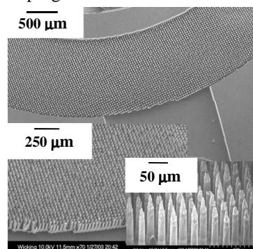
**Figure 3.** Scanning Electron Micrograph of silicon based evaporative structure
