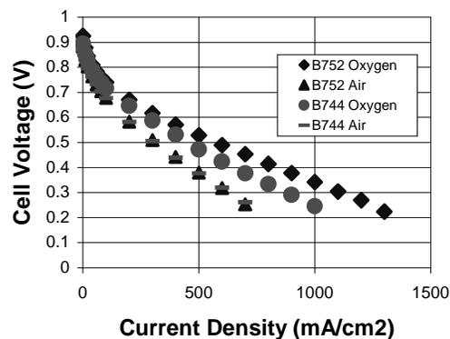
Fig 1. Active Area = 6.25 cm<sup>2</sup>, Cell Temp. 120°C, 35%RH, ambient pressure, catalyst loading: cathode 0.45mg/cm<sup>2</sup> Pt/C (Tanaka Kikinzoku Kogyo, Japan), anode 0.3 mg/cm<sup>2</sup> Pt-Ru/C(Tanaka Kikinzoku Kogyo, Japan).
