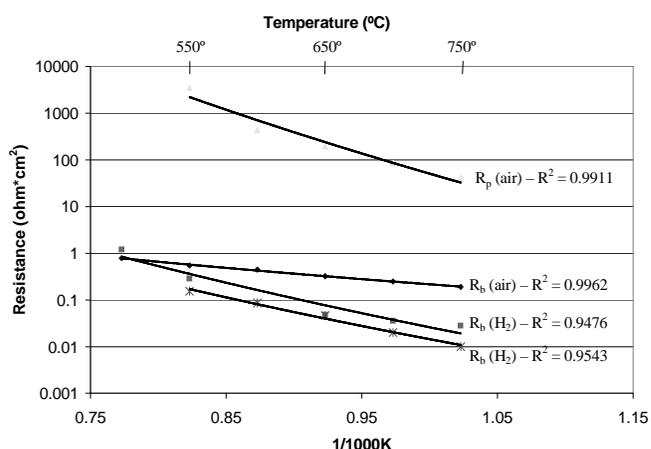
**Figure 3** – Log of area-specific polarization and bulk resistance values versus inverse temperature for the symmetric cell
