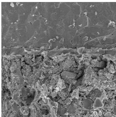
**Figure 1** – Cross-sectional view of GDC electrolyte and FeNiCr interconnect interface.
