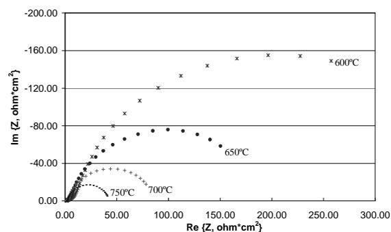
**Figure 2** – Impedance spectra for symmetric cell tested in air without DC polarization from 600°C -750°C
