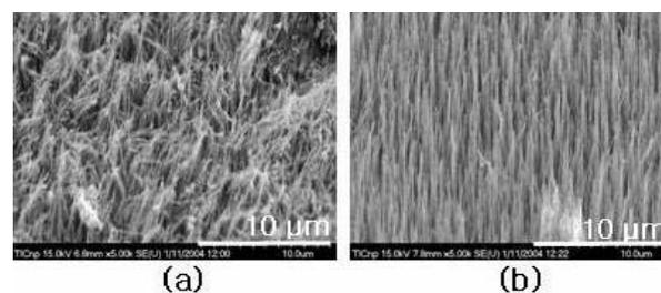
Fig. 2. SEM images of CNTs grown by PECVD at 650°C for 15 min on the sample of (a) unannealed, (b) annealed at 800°C for 50 sec.
