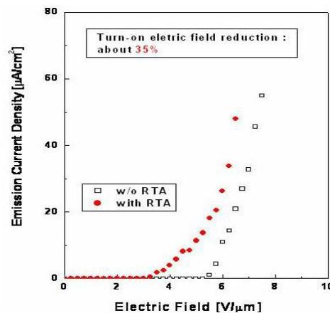
Fig. 3. Comparisons of field emission characteristics of CNTs grown with RTA treatment and as-grown CNTs.
