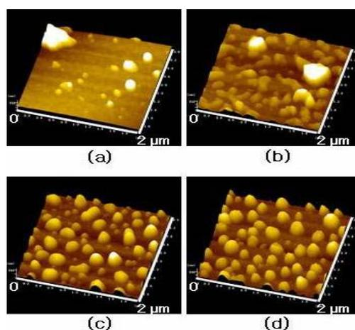
Fig. 1. AFM images of Ni islands formed by RTA treatment at various temperature. (a) unannealed, (b) 700°C, (c) 800°C, and (d) 900°C.
