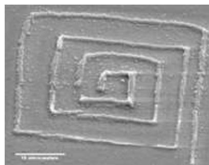
**Figure 2.** SEM image of MPE-photocrosslinked cyt *c* structure prepared on an ITO electrode. Scale bar is 10  $\mu\text{m}$ .
