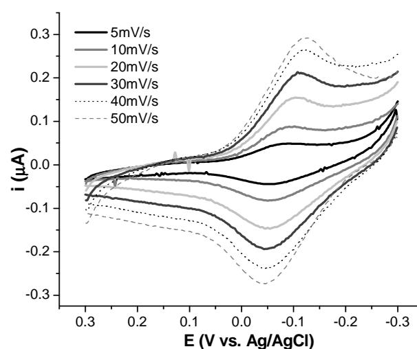
**Figure 3.** Cyclic voltammograms of photocrosslinked cyt *c* on an ITO electrode.
