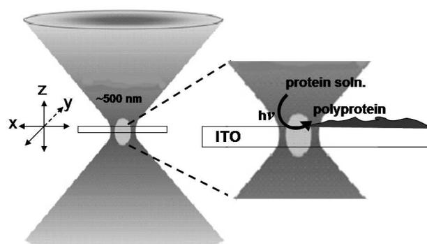
**Figure 1.** Multiphoton excitation (MPE) fabrication of photocrosslinked protein structures. MPE is contained within the volume depicted by the light grey oval (~1 fL).
