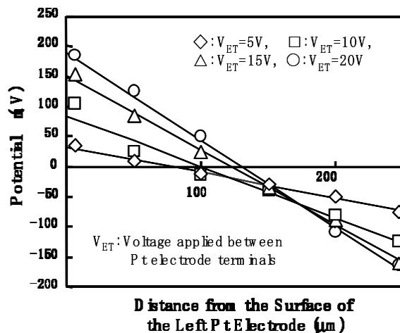
Fig.2 Potential gradients between Pt electrodes
