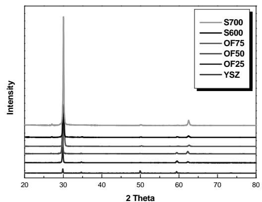
Fig 2. X-ray diffraction patterns of YSZ layers, which have been prepared under various temperature and oxygen flow rate conditions.
