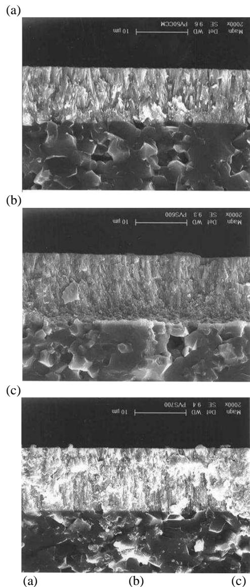
Fig 1. SEM photographs of YSZ electrolyte film deposited on porous substrate. The substrate temperature during deposition was maintained at (a) 873 K, (b) 973 K, and (c) 1073 K respectively.
