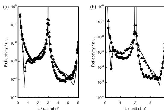
Fig. 1 The specular rod profiles at (a) Au(111) and (b) Au(100). Circles and triangles were measured at 0 V and +1.40 V, respectively. Solid lines are the calculated curves.
