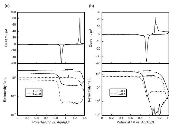
Fig. 2 Cyclic voltammograms and potential dependence of X-ray scattering intensity at (a) Au(111) and (b) Au(100). Solid and dotted lines are L = 0.7 and L = 0.8, respectively, at Au(111) and are L = 0.4 and L = 0.5, respectively, at Au(100).
