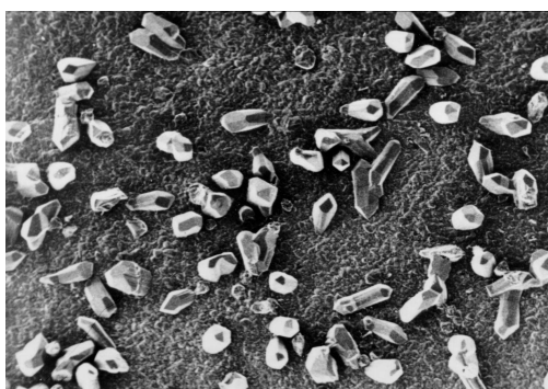
Fig. 3. Microstructure of a niobium stannide (a) before and (b) after exposing at 800 K in the E- \text{K}_2\text{NbF}_7 melts ( \times 100 ).
