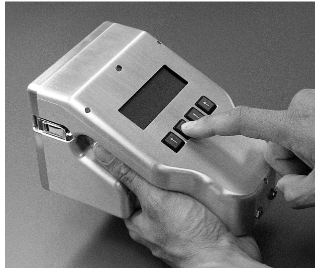
Figure 1: The hand Portable capillary electrophoresis device, \mu Chemlab.
