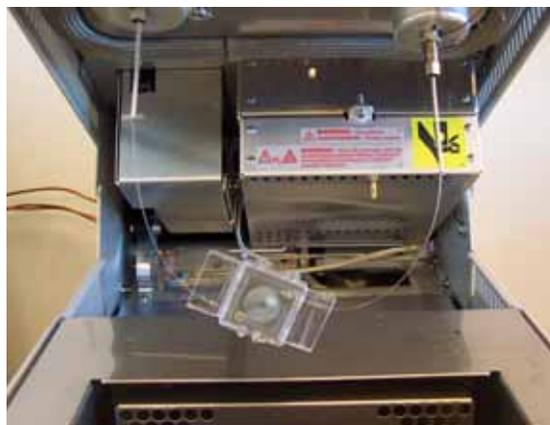
**Figure 1.** Miniature parylene GC column installed in conventional GC (HP 6850).
