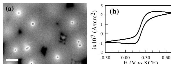
**Fig. 2** (a) The SEM image of a MWNT nanoelectrode array embedded in SiO<sub>2</sub> matrix. The scale bar is 500 nm. (b) The cyclic voltammetry of the MWNT nanoelectrode array in 1.0 mM K<sub>4</sub>Fe(CN)<sub>6</sub> and 1.0 M KCl at a scan rate of 20 mV/s.
