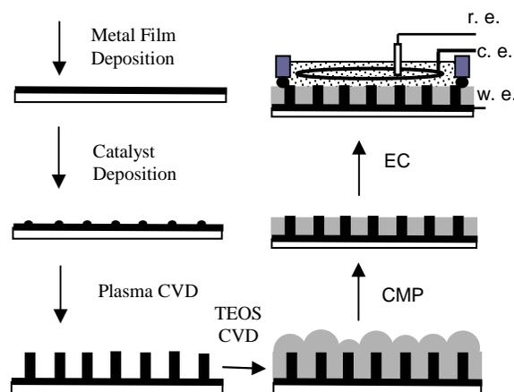
**Fig. 1** The procedure for fabricating the MWCNT nanoelectrode array and the setup for electrochemical characterization.
