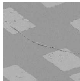
Figure 1. Immobilization of the avidin-coated nanotube on biotinylated thiol-SAM/Au surfaces. [Matsui, H.; Porrata, P.; Douberly, G. E., Jr., Nano Lett. 1 , 461, (2001)].
