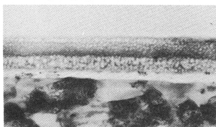
Figure 2. T.E.M. of ultramicrotomed section of electropolished Al foil anodised at 50V. for 1hr. in anhydrous molten \text{LiNO}_3\text{-KNO}_3 eutectic at 140^\circ\text{C} .
