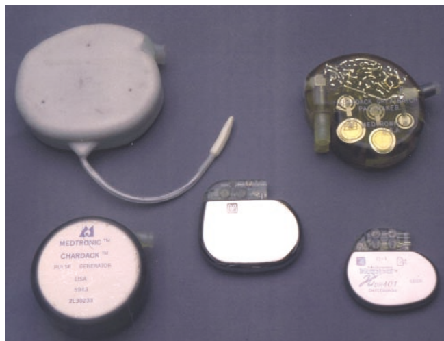
Fig. 1. Battery-powered implantable devices have been in use for over 40 years, and the first successful cardiac pacemaker was implanted in 1960. Shown here is a "history of pacing" — from the first implantable (upper left) to the Kappa DR 401 (lower right). Image courtesy of Medtronic.
