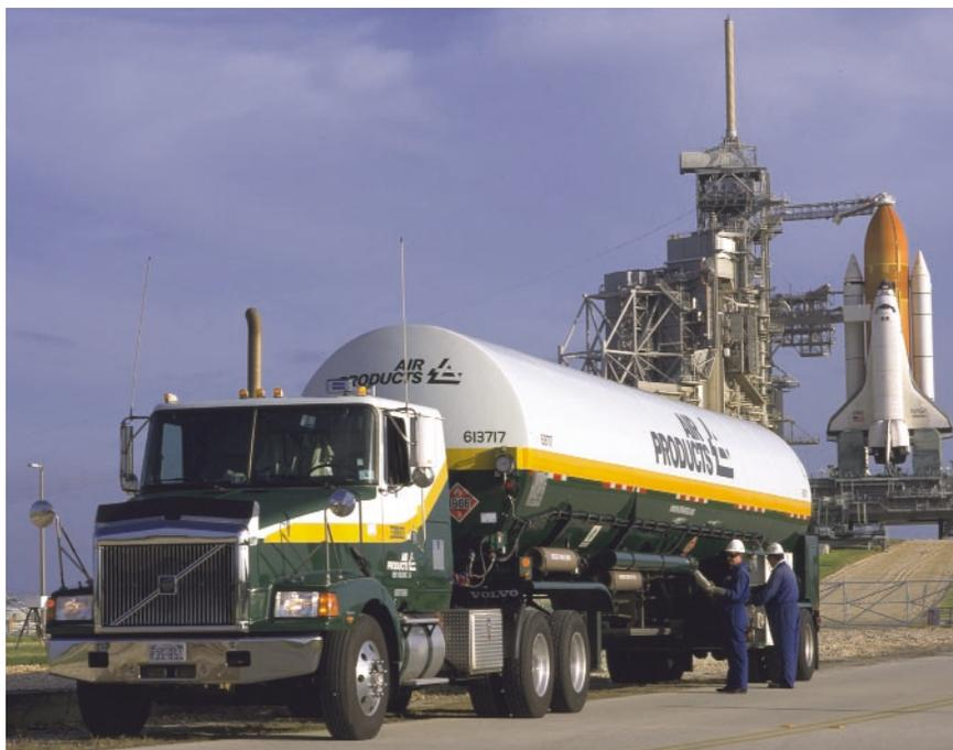
Fig. 3. Supplying H<sub>2</sub> fuel for a space shuttle at Kennedy Space Center. Photo courtesy of Air Products and Chemicals, Inc.
