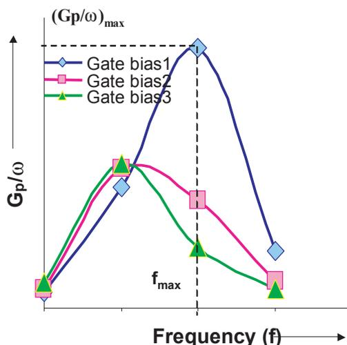
Fig. 4.  $G_p/\omega$  vs.  $\log(f)$  plots for different gate biases in the depletion regime.  $D_{it}$  is computed from the highest peak of the plots.
