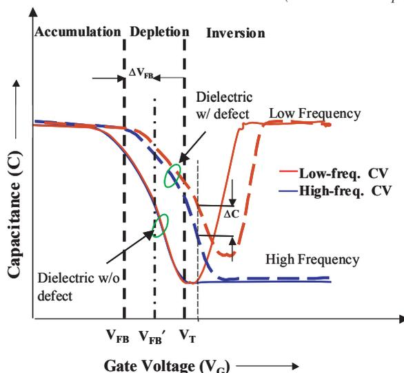
Fig. 2. High-frequency (hf) and low-frequency (lf) capacitance-voltage (C-V) characteristics of MIS structure for dielectric films with and without (ideal) defects are shown. Flatband voltage shift of hf C-V,  $\Delta V_{FB} = (V_{FB}' - V_{FB}) > 0$  indicates negative charge trapping. For a film with defects, stretch-out of hf C-V, and offset in capacitance,  $\Delta C$ , in between hf and lf C-V indicate the presence of interface traps.
