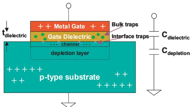
Fig. 1. A metal/insulator/semiconductor (p-type) (MIS) structure is shown that is used extensively to characterize dielectric films. Dielectric/semiconductor interface traps and bulk traps are shown. For positive gate bias, semiconductor and metal gate act as cathode and anode, respectively, whereas for negative gate bias, the opposite holds. The equivalent circuit of the series capacitance of dielectric and depletion capacitances is also provided.
