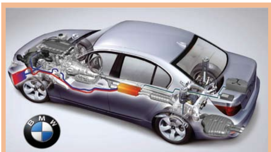
FIG. 2. Conceptual design of thermoelectric generator producing electricity from waste heat in the engine exhaust. Copyright BMW, reprinted by permission.
