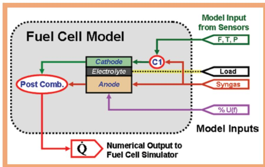
Fig. 4. Diagram of the Hyper facility real-time fuel cell model.
