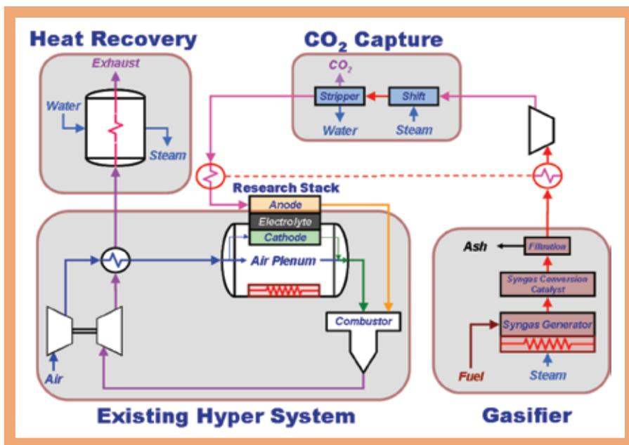
Fig. 6. Proposed modifications to the Hyper facility for expanding the scope of hybrid system exploration.
