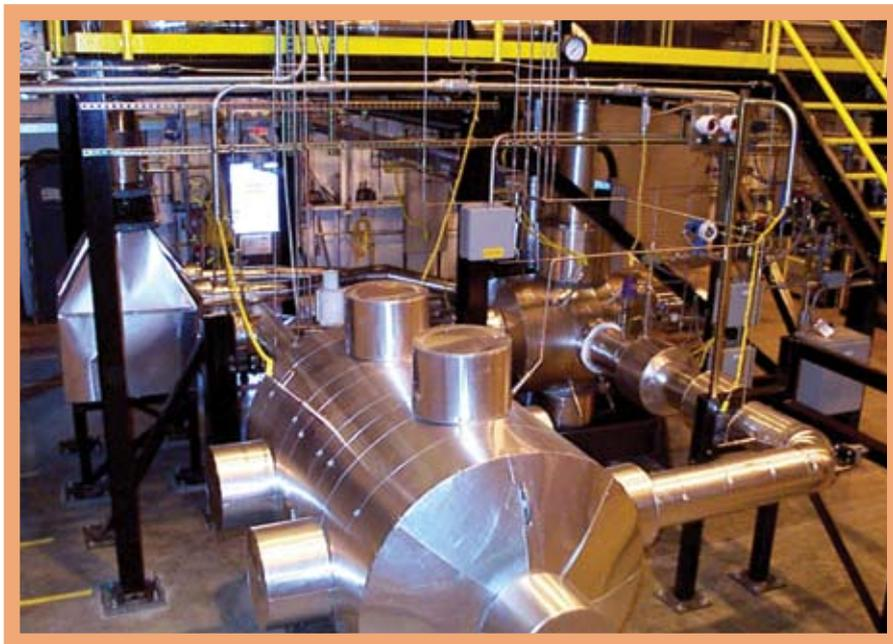
Fig. 3. A photograph of the Hyper facility at NETL (the cathode volume is shown in the foreground).
