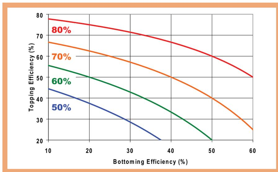
Fig. 5. Total system efficiency as a function of topping and bottoming cycle efficiencies.
