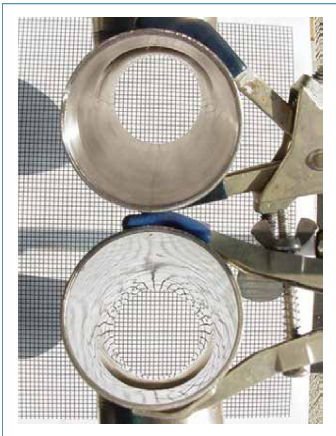
Fig. 3. 316SS fitting surface before (top) and after (bottom) pulse reverse electropolishing in an NaCl-NaNO 3 electrolyte.
