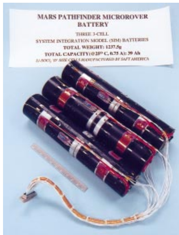
Fig. 5. (right) Sojourner Rover. Li-SOCl 2 Batteries. (Photo courtesy of Jet Propulsion Lab.)
