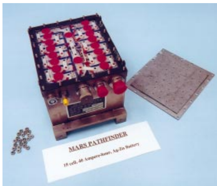
Fig. 4. (above) Mars Pathfinder. Silver-Zinc Battery. (Photo courtesy of Jet Propulsion Lab.)
