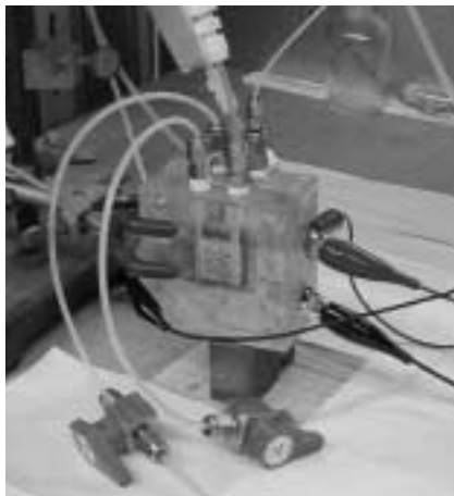
Fig. 3. Rectangular cell for CO 2 reduction with 2 x 2 cm gas-diffusion cathode.
