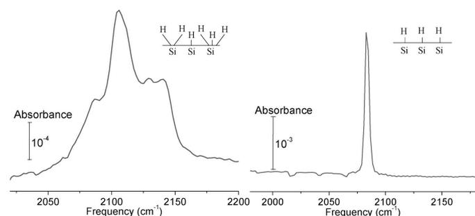
Fig. 1 Infrared absorption spectra of (left) atomically rough H/Si(100) characterized by a broad and structured spectrum representing several hydride termination (mono-, di-, trihydrides) and (right) atomically smooth H/Si(111) surfaces defined by a sharp, resolution limited feature polarized perpendicular to the surface.
