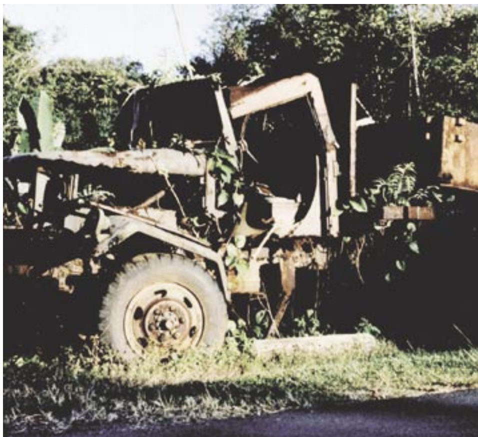
Fig. 4. Photograph of badly corroded truck after unknown years of marine atmospheric exposure. Photo was taken in Hawaii while attending a meeting of The Electrochemical Society.
