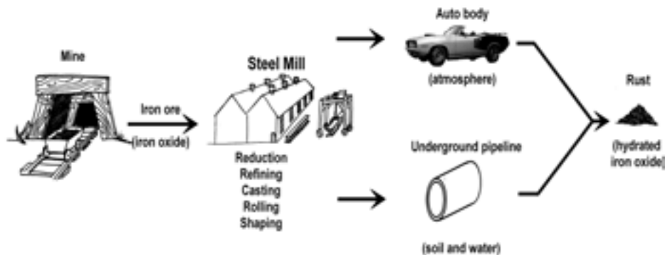
Fig. 1. Why does steel corrode?
