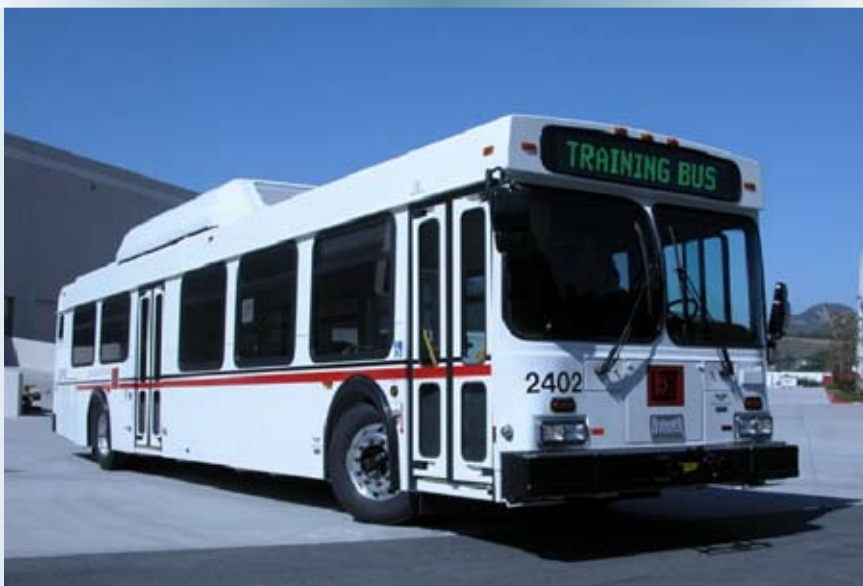
Fig. 2. Hybrid city transit bus that uses an electrochemical capacitor energy storage system. Typical charge/discharge periods may be forty seconds in this application with continuous 16-hours-per-day operation (>1000 charge/discharge cycles each day). (Photo courtesy of ISE Corporation.)
