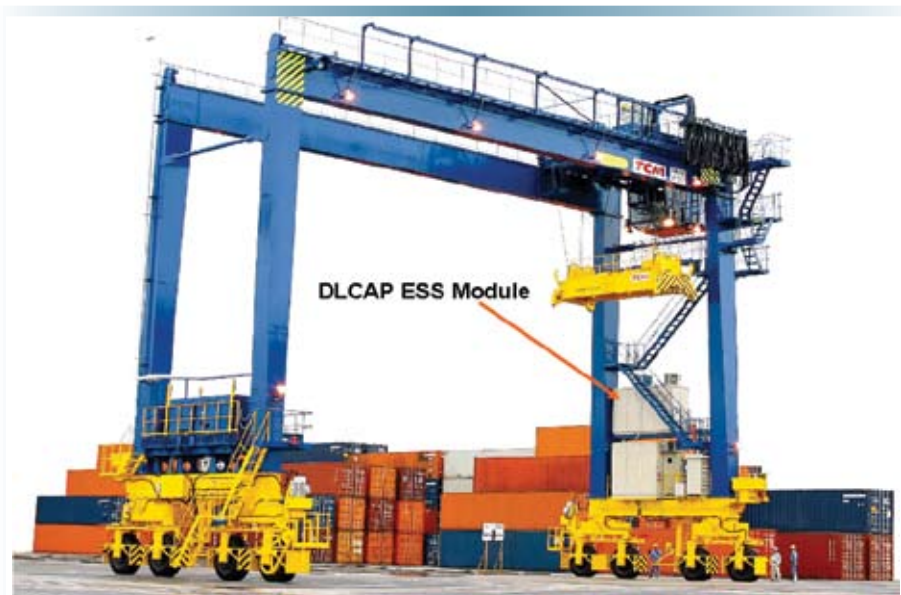
Fig. 1. Hybrid diesel/electric rubber tired gantry crane with an electrochemical capacitor energy storage system. This crane is used for loading and unloading container ships. The capacitor system captures and stores regenerative energy during load lowering that is then used to help raise the next load, resulting in improved efficiency and greatly reduces air emissions. (Photo courtesy of Nippon Chemi-Con Corporation.)
