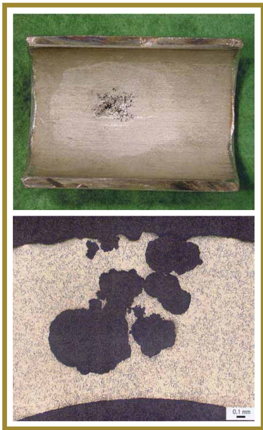
Fig. 1. Pitting corrosion of a stainless steel pipe, showing growth of pits under the metal surface. Courtesy of Intertek-CAPCIS
