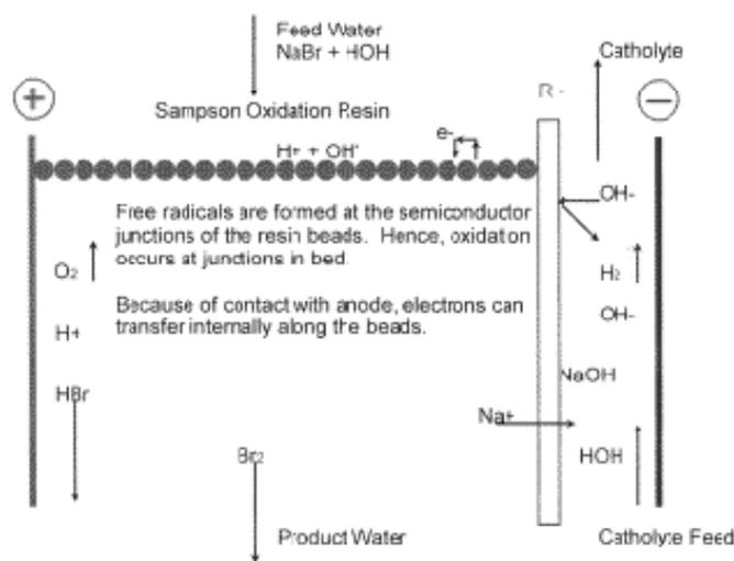
Fig. 1. Sampson Oxidation Membrane Cell. Depicts bromine production although chlorine dioxide is generated in a similar manner. Figure courtesy of Halox Technologies Corporation (Bridgeport, CT).
