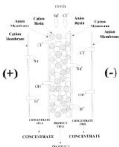
Fig. 2. Schematic of plate and frame electroionization cell. Softened water is removed of  $\text{Na}^+$  and  $\text{Cl}^-$  to make high purity water. Courtesy of US Filter (Lowell, MA.)
