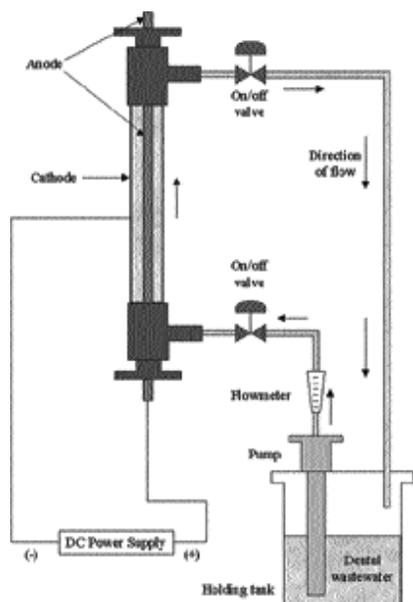
Fig. 4. Electrocoagulation process for removing mercury amalgam from dental wastewater.
