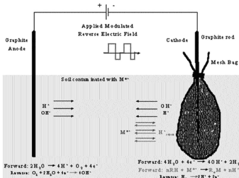
Fig. 5. Enhanced electrokinetic system. pH front is eliminated so metal cations transport to the cathode and are collected in the ion-exchange resin. Figures 4 and 5 courtesy of Faraday Technology, Inc. (Clayton, Ohio).
