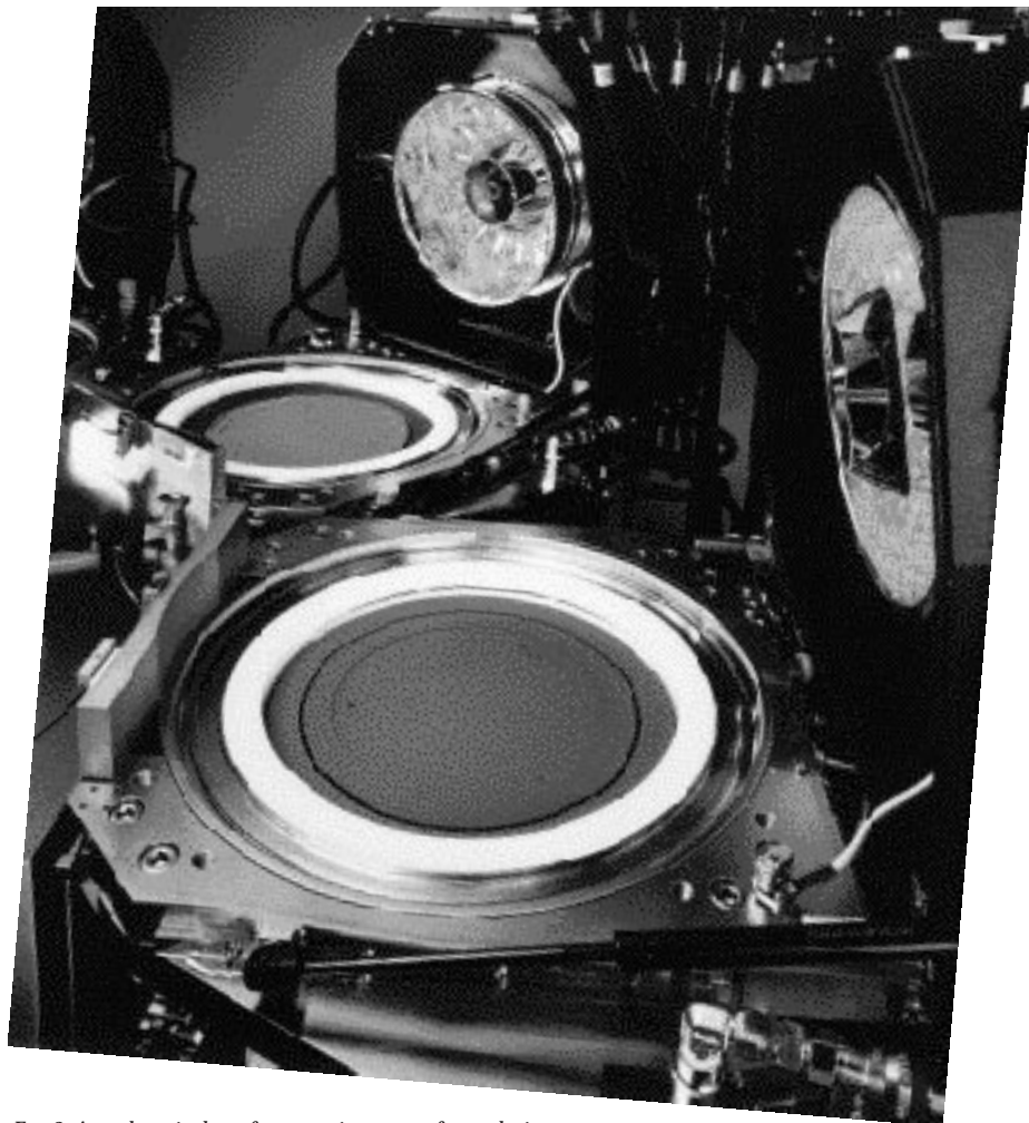
FIG. 3. A modern single-wafer processing system for producing epitaxial silicon films. This equipment can process wafers as large as 300 mm in diameter. (Photograph courtesy of Applied Materials)
