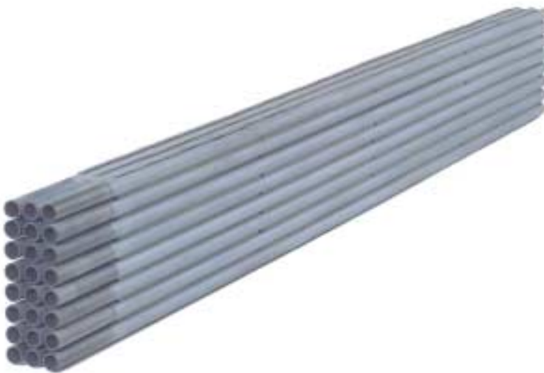
Fig. 4. Photograph of a three-in-parallel and eight-in-series cell bundle.
