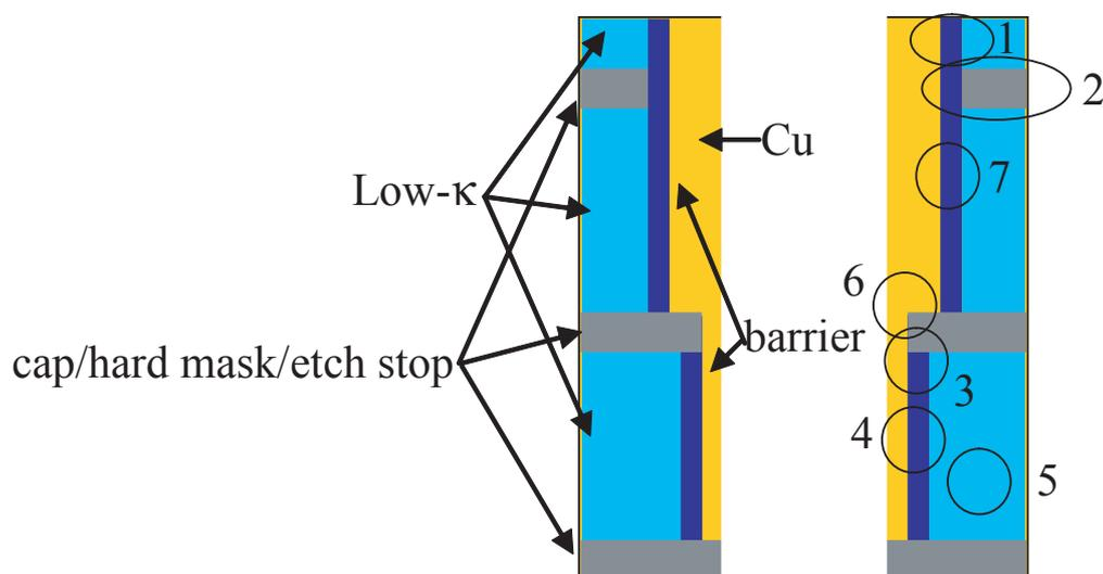
FIG. 3. Schematic of integration issues associated with low-k processing.<sup>15</sup>
