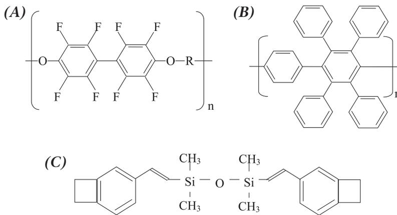
FIG. 2. Schematic of low-*k* polymers. (A) FLARE™, (B) SiLK™, and (C) Cyclotene™.
