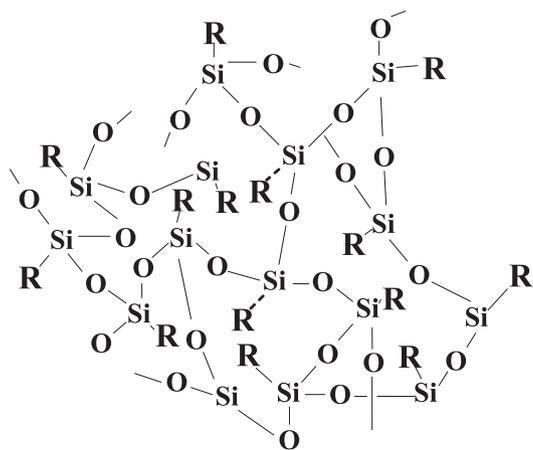
FIG. 1. Schematic representation of OSG structure. In MSQ, R = CH<sub>3</sub>; for HSQ, R = H; for FSG, R = F; and for HOSP, R = both CH<sub>3</sub> and H. These compounds can be spin-on or CVD/PECVD dielectrics.
