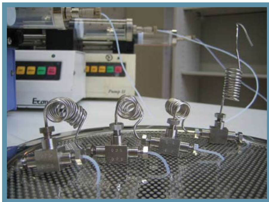
Fig. 1. An integrated microflow reactor system consisting of four micromixers and four microtube reactors.
