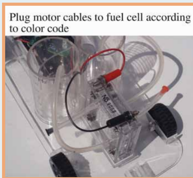
FIG. 8. Connection of the fuel cell to the electric motor.
