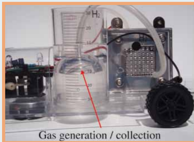
FIG. 6. Example of gas generation in the PEM electrolyzer.
