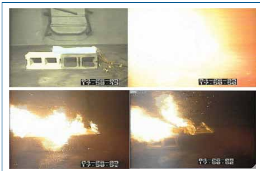
FIG. 4. Failure sequence of a commercial Li-ion battery (clockwise from upper left).
