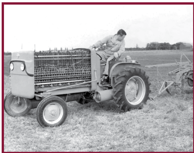
FIG. 1. 15 kW AFC-powered tractor of Allis-Chalmers. (From the National Museum of American History, Science Service Historical Images Collection, courtesy of Allis-Chalmers.)
