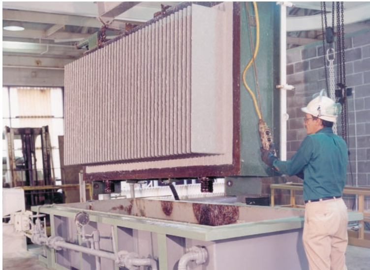
FIG. 3. Tephram Diaphragm on a Glanor V-1244 Electrolyzer Cathode.
