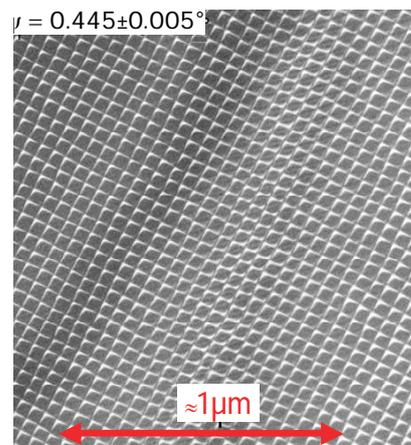
Fig. 10. A two-dimensional dislocation array obtained by bonding two Si (100) wafers with a small twist angle  $\Psi$  between the top and bottom wafer (from Ref. 54).
