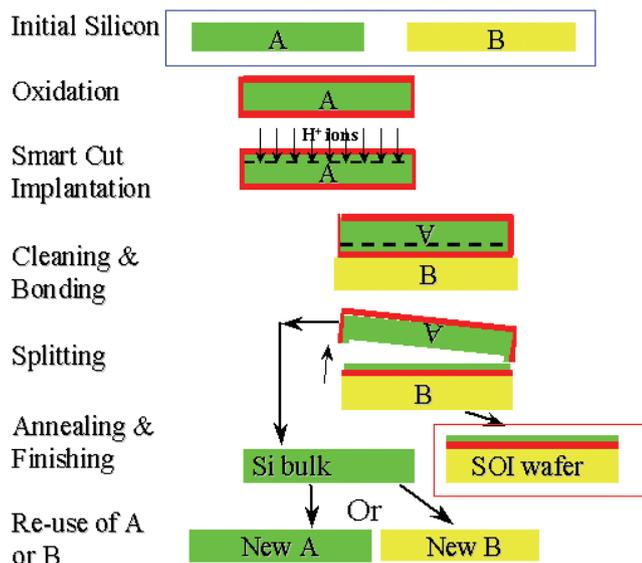
**Fig. 2.** A schematic process flow for SOI wafer fabrication by Smart Cut™ technology.
