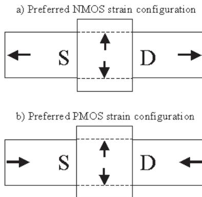
**Fig. 5.** Ideal strain configurations for n-MOS and p-MOS transistors (after Ref. 42).
