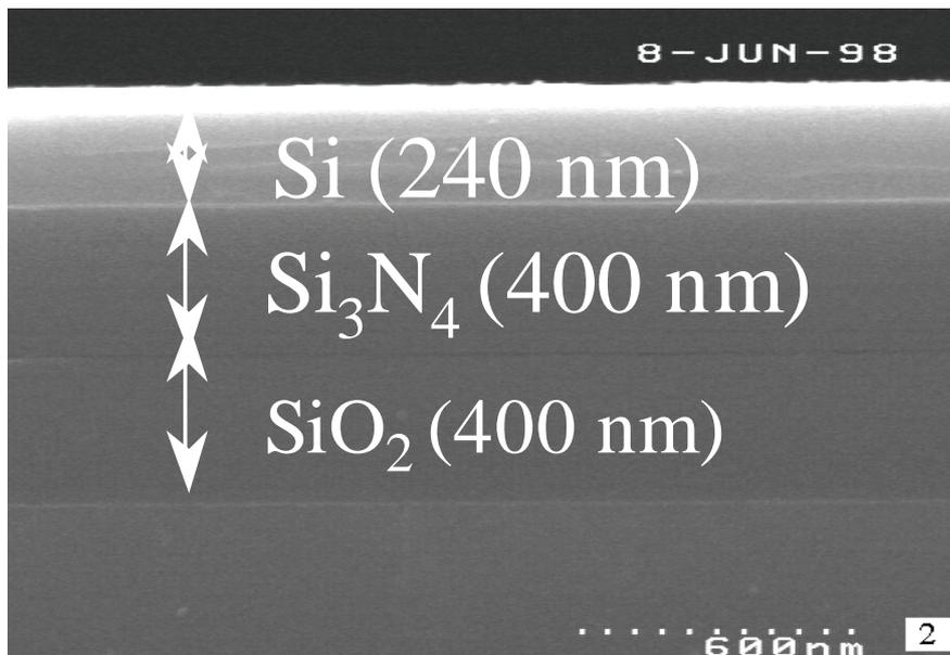
Fig. 9. SEM micrograph of a composite nitride/oxide buried dielectric under a silicon film.
