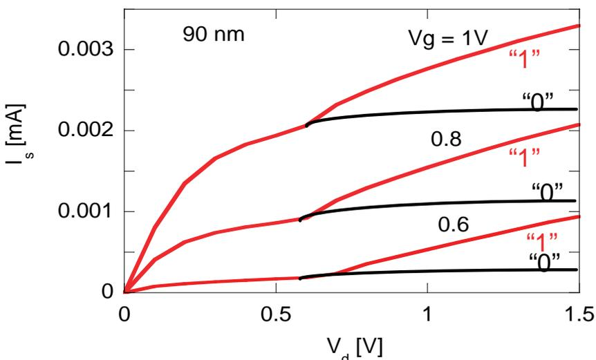
Fig. 11. Electrical I-V curves of a floating-body SOI transistor depend on the charge that is present in the body. This can serve to store memory bits (from Ref. 57).
