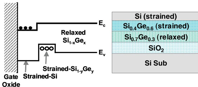
**Fig. 8.** Schematic layer structure and band diagram for a dual channel device that is based on strained Si deposited on top of strained SiGe (after Ref. 43 and 44).
