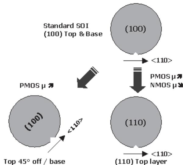
**Fig. 3.** Crystalline plane orientations and directions within the planes that improve electron and/or hole mobility in Si MOSFETs.
