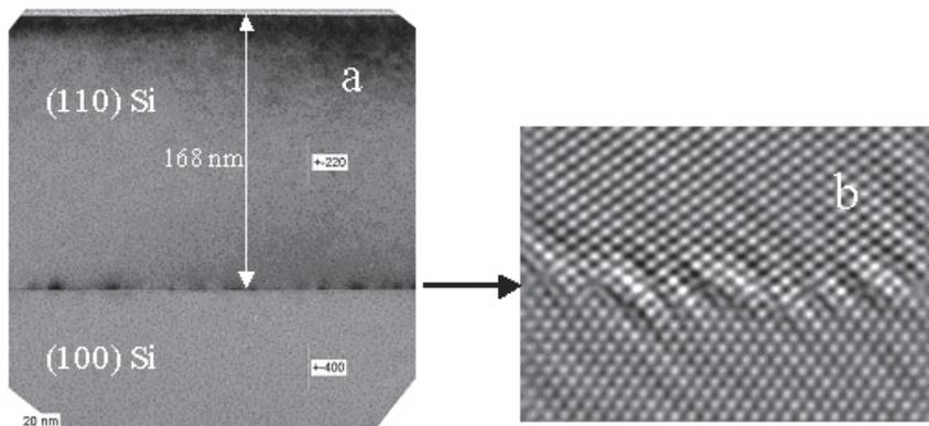
**Fig. 4.** (a) XTEM image of the DSB wafer and (b) XRTEM image of the bonding interface (from Ref. 31).
