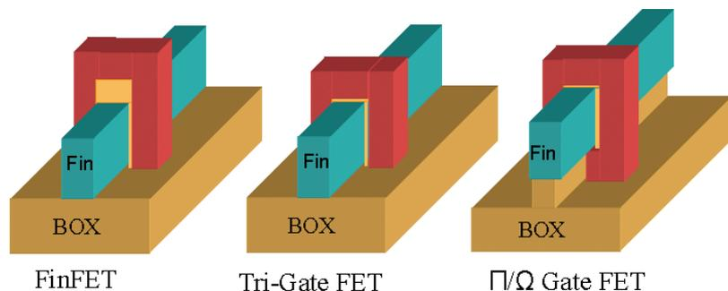
Fig. 12. Three configurations for a Fin-based multi-gate transistor.
