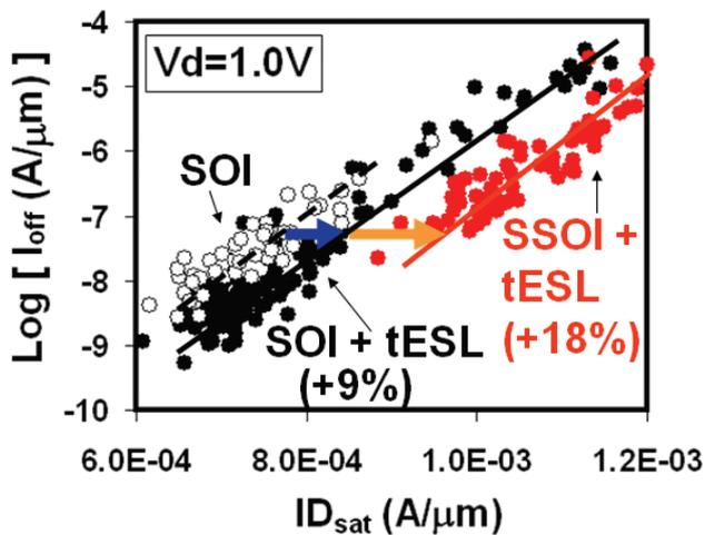
**Fig. 6.** Drive current  $ID_{sat}$  vs.  $I_{off}$  for n-MOS devices with various stressors (from Ref. 42).
