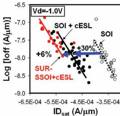
**Fig. 7.** Drive current  $ID_{sat}$  vs.  $I_{off}$  for p-MOS devices with various stressors (from Ref. 42).
