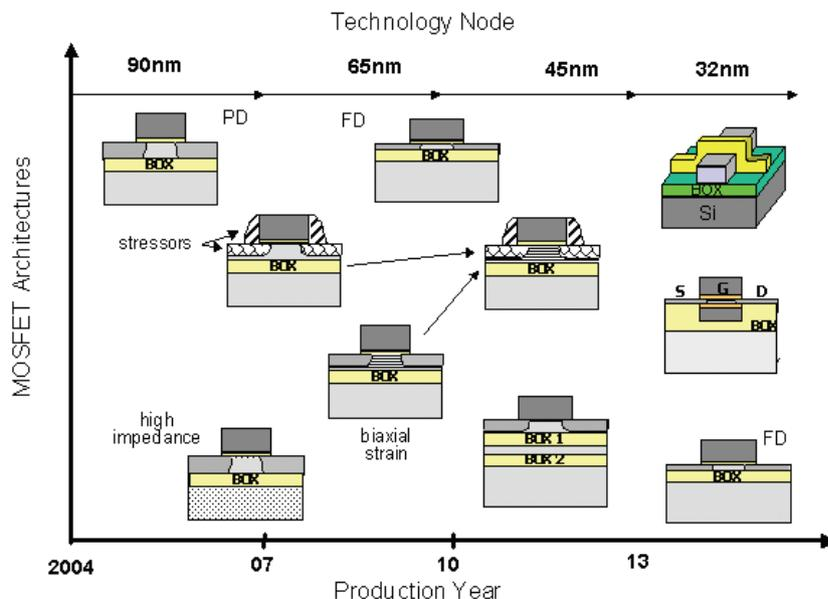
Fig. 1. Device architectures that are either already in use or are anticipated in future technology nodes.
