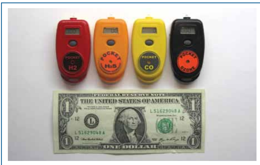
Fig. 5. A family of “Pocket” smart sensor systems measuring a range of individual gases. (Courtesy KWJ Engineering Inc. 15 )
