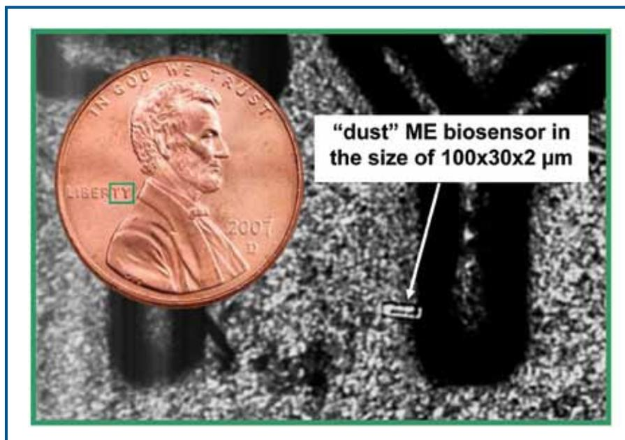
**Fig. 3.** Scanning electron micrograph comparing the size of a ME biosensor with the Y in "LIBERTY" on a penny. The biosensors are microelectronically fabricated and are smaller than a particle of dust. The biosensors require no on-board power and their cost is less than 1/1000 of a cent each when fabricated in large numbers.
